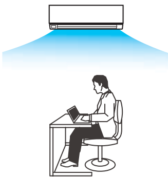
Ideal air flow discharge on cooling mode
