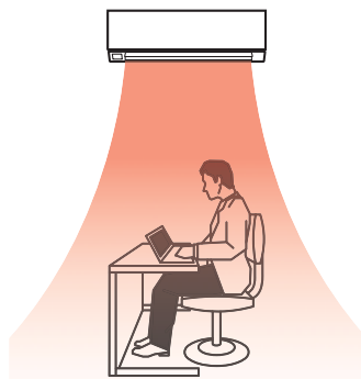
Ideal air flow discharge on heating mode
